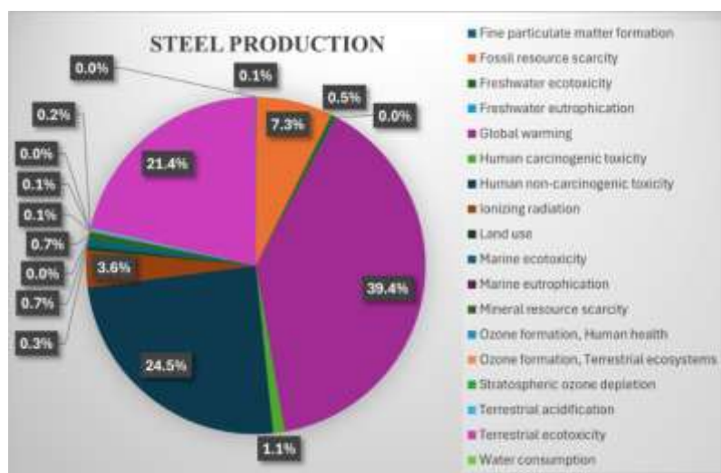
Fig. 5.5 Percentage Contribution of Environmental Impact Categories in Steel Production
