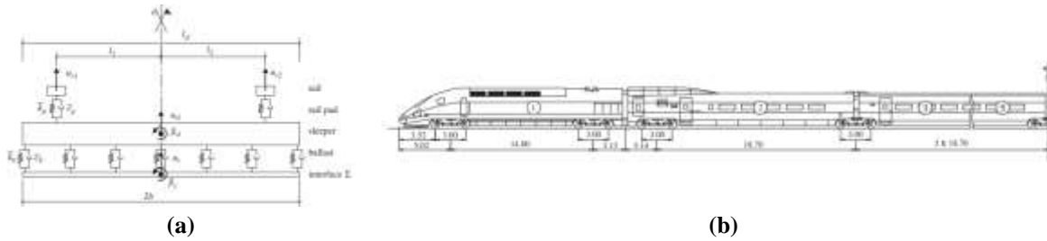
Fig. 21 (a) Cross section of a ballasted track model (b) The configuration of the Thalys HST[52]
