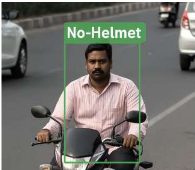
Fig. 02 – YOLOv8 detection output showing No-Helmet classification.
