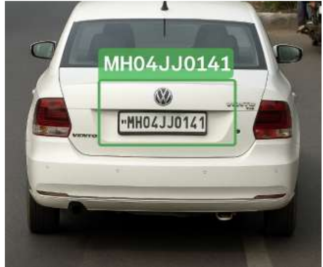
Fig. 03 – OCR output from a traffic video frame with extracted plate text.
