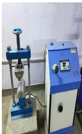
Figure 3(a): Split Tensile Test
