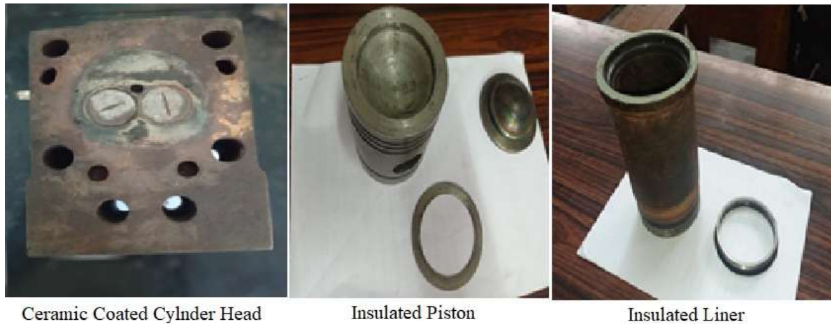
Fig.1 Photographic views of Heat Loss diesel engine with different degree of insulation
