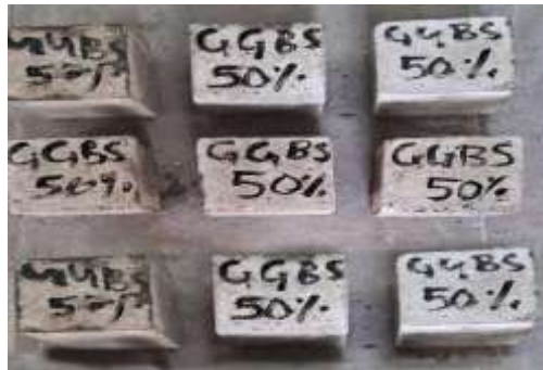
Fig.4.1 Concrete Cube Specimen (150mm×150mm×150mm)
