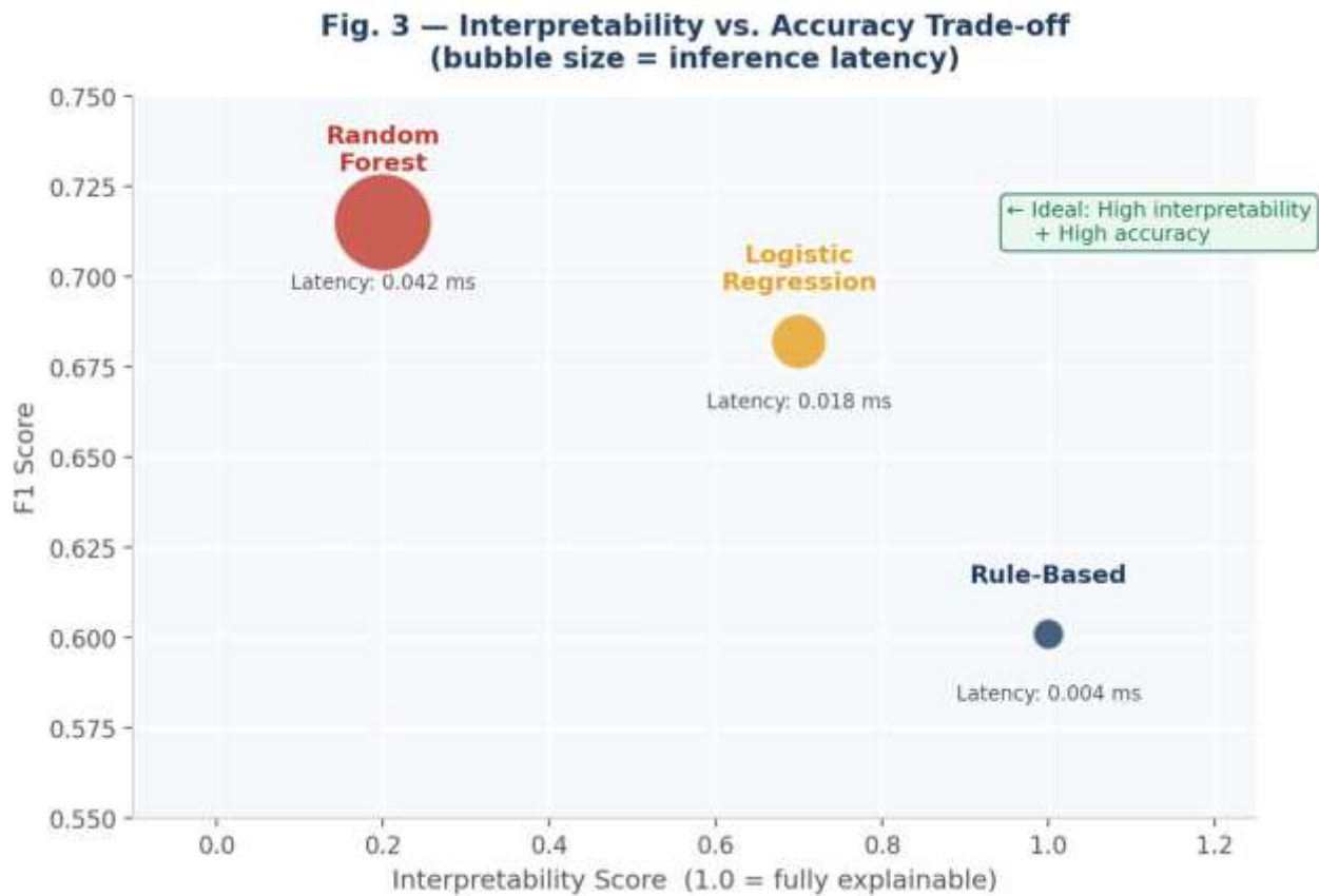
Fig. 3. Interpretability vs. Accuracy Trade-off. Bubble size represents inference latency; the ideal method occupies the upper-right corner (high interpretability, high accuracy).
