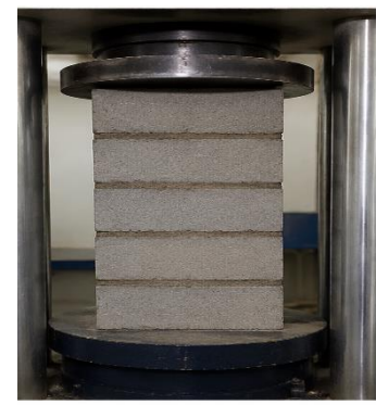
Fig. 1 c) Fly ash brick masonry (5 layers)
