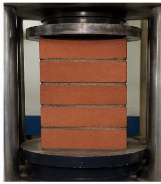
Fig. 1 b) Machine-made red clay brick masonry (5 layers)
