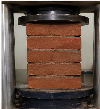
Fig. 1 a) Handmade red clay brick masonry (5 layers)
