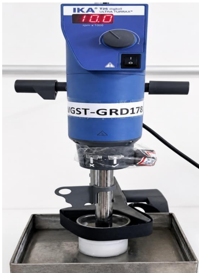
Fig. 2: Experimental setup for K-SLN preparation by modified high-speed homogenization.
