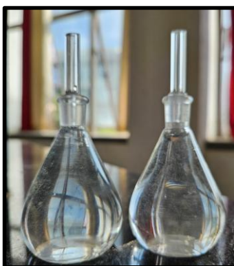
Fig. 12: Determination of specific gravity using pycnometer.
