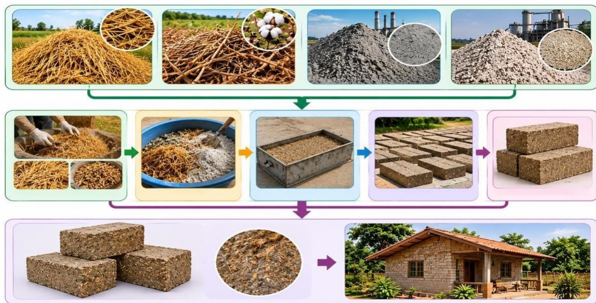
Fig.1 Conceptual Illustration of Hybrid Bio-Brick Production Using Agricultural Waste and Industrial By-Products for Sustainable Rural Housing.
