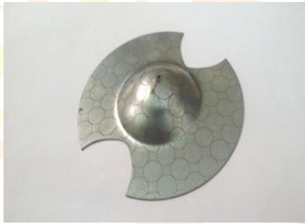
Fig. 6 Identification of failure locations for Nakazima test
