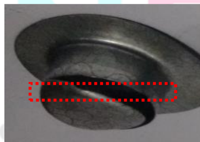
Fig. 8 Identification of failure locations for cup drawing test
