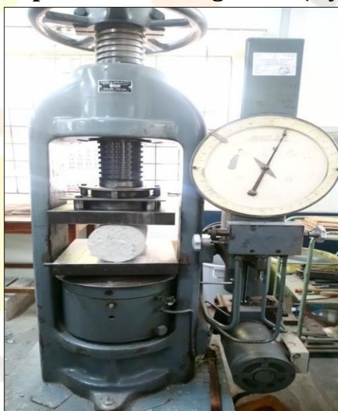
Fig. 4.3 Split tensile strength test (Cylinder)
