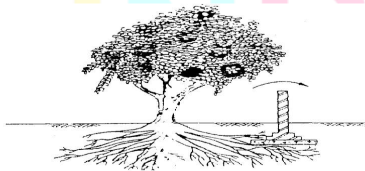
Figure 1.6 Roots of fast-growing tree under the foundation of compound wall may topple down the wall.
