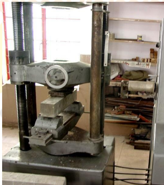
Fig.4.5 Flexural strength test
