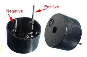
A buzzer, a simple yet versatile electroacoustic device, holds a pivotal role in numerous applications across various fields. At its core, a buzzer converts electrical energy into sound waves, producing audible alerts or signals. The design and functionality of buzzers have evolved over time, catering to diverse needs in industrial, commercial, and consumer contexts.
